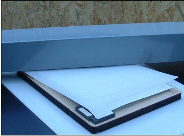
Test the cutting result and in small steps increase the cutting pressure with the setting screws until the machine cuts the whole shape perfectly.
